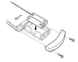
Use a Philips driver to remove the cover from the bottom of the remote control, and pull out the battery case. Insert two AA batteries in the correct  $\oplus/\ominus$  orientations, reinsert the case and close the cover.
